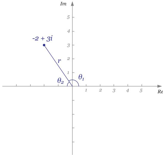
Figure 9:  $z = -2 + 3i$  plotted on an Argand diagram
