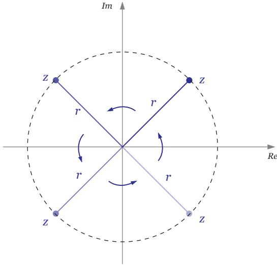
Figure 15: The locus traced out by  $|z| = 4$  on an Argand diagram
