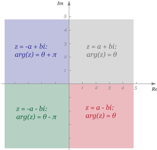
Figure 10: Rules for calculating  $\arg(z)$  in different quadrants
